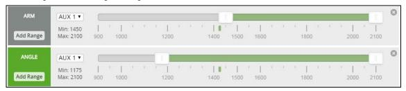
6. Turn on the transmitter and move to the AUX. Channels interface, Set "SWA" or "SWB" switch etc. for CH5 to ARM/DISARM the motor, Take FLYSKY I6 as an example.
